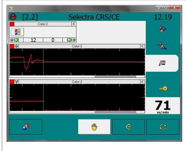
At the end the **error histogram screen** is more powerful than before granting the operator to control a longer period of time. Moreover it shows length and side errors together with the machine speed variation histogram.
