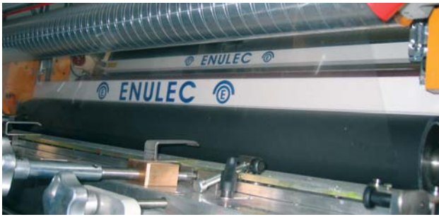
Enulec ESA unit installed in a gravure print station.
